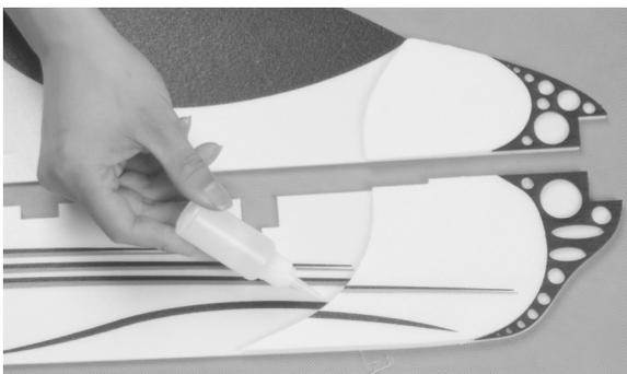
Glue the foam strengthen slice to the head of fuselage side board.
