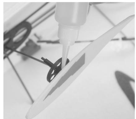
Install wheel covers on the chock beside the wheel. Screw one more chock outside of the cover, glue it.
