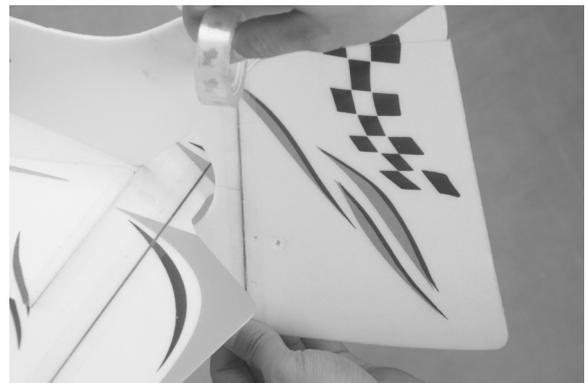
Hinge the rudder to the back of the fuselage, using the same techniques that you used to hinge the Elevator to the stabilizer.
