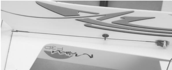
Center the elevator and rudder servo, then attach the servo arm to the servo.
