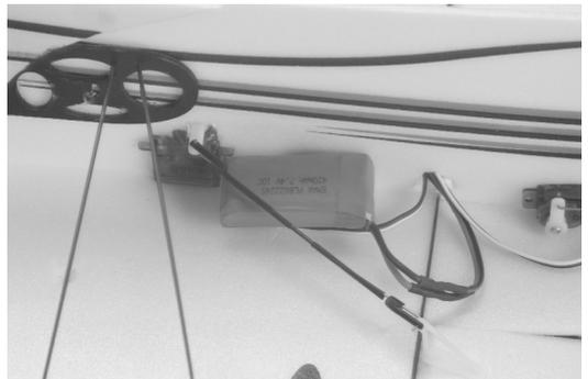
Install your battery into the battery compartment, using a piece of hook and loop material.
