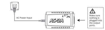
2) The LEDs will begin to blink in an alternating pattern. This means the charger is ready for use. Place the battery is a flame-resistant charging device like a Common Sense RC® Lipo Safe Bag. Plug the balance leads of your battery into the output port that exactly matches the balance connector on your battery.
