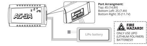
3) After the battery has been connected, the LEDs on the charger will blink to indicate the charge level of the battery.
