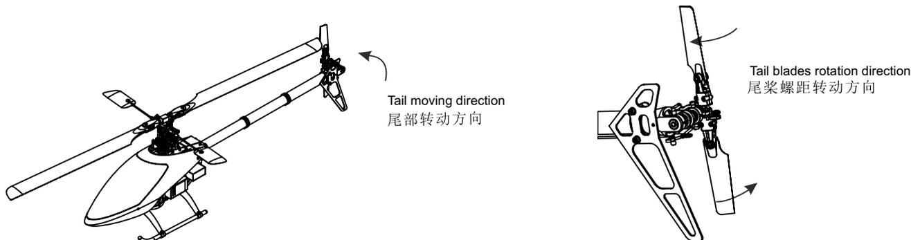
5. Check that main blades, paddles and tail blades are installed in the right direction.
