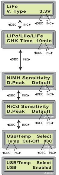
The screen displays the nominal voltage of Lithium battery. There are three kinds of Lithium battery; LiFe(3.3V), Lilo(3.6V) or LiPo(3.7V). This is very important so you have to check the battery carefully and set it up correctly. If it is different from correct value the battery can explode during charge process.
