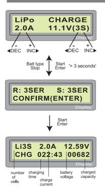
The left side of the first line shows the type of battery you select at the users setting. The value on the left side of second line sets a charge current and the value on the right side of second line sets the voltage of the battery pack.
