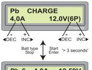
Set up the charge current on the left and the nominal voltage of the battery on the right. The charge current ranges from 0.1 to 5.0A and the voltage should be matched with the battery being charged.
