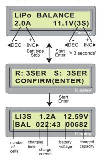
The value on the left side of second line sets a charge current and the value on the right side of second line sets the voltage of the battery pack.
