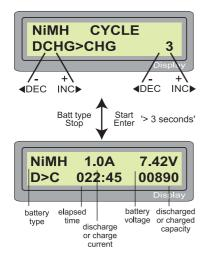
Set the sequence on the left and the number of cycle on the right. You can use this function for balancing, refreshing and break-in the battery. To avoid rising temperature of the battery, there will a brief cool-off period that already fixed at 'User setting' after each charge and discharge process. The cycling number ranges from 1 to 5.
