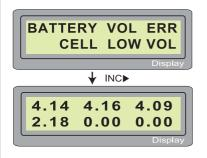
The processor found that the voltage of one of the cell in the Lithium battery pack is too low.
