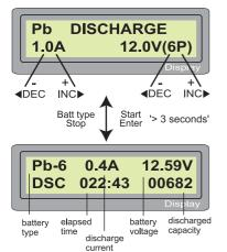
Set discharge current on the left and final voltage on the right. The discharge current ranges from 0.1 to 1.0A.
