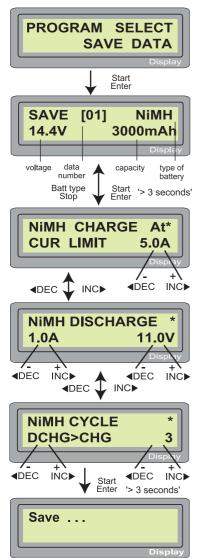
The parameter value setting up in this screen does not affect charge or discharge process. They only represent the specification of the battery. The following screens will automatically be displayed exactly matched with the battery type you set up. The example shows the battery pack of NiMH, 12 cells and 3000mAh of capacity.
