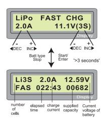
You can set up the charging current and the voltage of the battery pack being charged. As you press Start button the voltage confirmation will be displayed. And then, if you confirm the voltage and current, press Start Enter button again to start charging.
