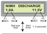
Set discharge current on the left and final voltage on the right. The discharge current ranges from 0.1 to 1.0A and the final voltage ranges from 0.1 to 25.0V). To start the process, press Start key for more than 3 seconds.
