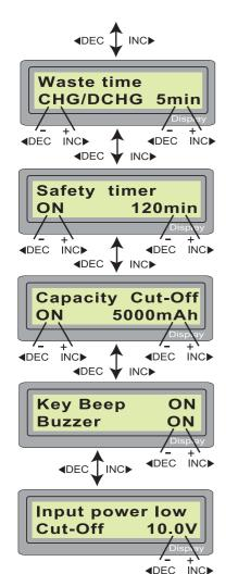
The battery is on the cyclic process of charge and discharge can often become warm after charge or discharge period. The program can insert a time delay to occur after each charge and discharge process to allow the battery adequate time to cool down before being subjected to the next process. The value ranges from 1 to 60 minutes.
